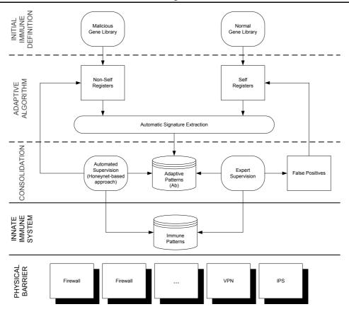
Figure 3. A three–layer architecture which combines traditional IDS concepts, data mining, honeynets and, just when strictly needed, the security expert supervision.
